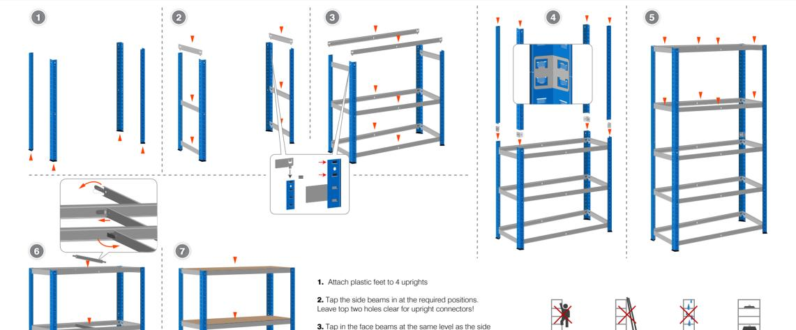
**4.** Attach the other 4 uprights to the top of the already assembled frame using the upright connectors.
