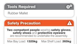
For maximum safety and stability, we recommend that the bay is fastened to a wall.
